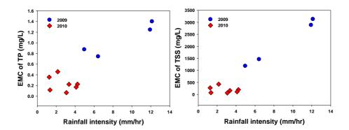
Figure 4. Comparison of EMC of TP and SS in the Naedong stream according to rainfall intensity
