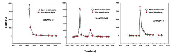
Figure 2. The removal efficiency of TSS by debris barrier during storm events
