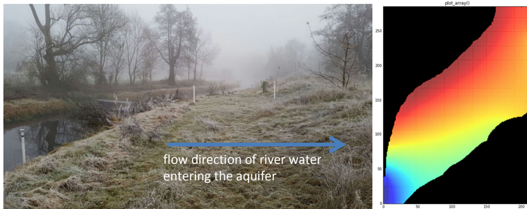
Figure 2. Right: Well gallery at River Erpe installed for taking alluvial groundwater samples. Left: MODFLOW model of subsurface water flow in alluvial bank (arrows show direction of flow; in black: aquifer boundary; colored grids represent groundwater heads from relatively high, in red, to relatively low, in blue).
