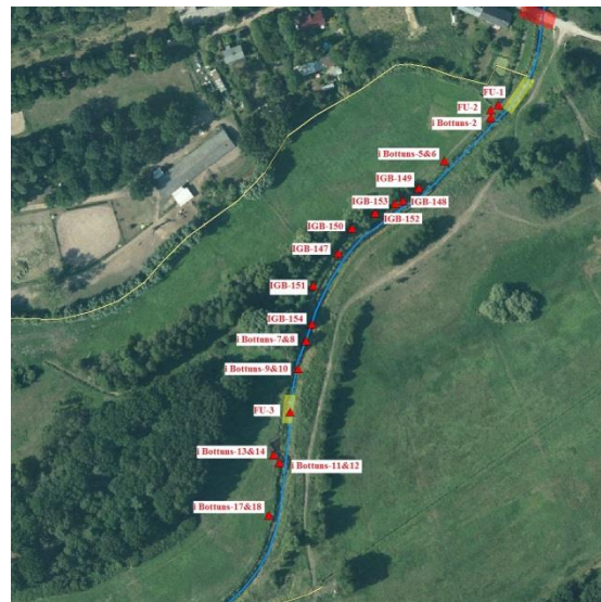
Figure 7: Temperature lances location
