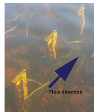
Figure 4. Passive samplers installed in flowing water and hyporheic sediments.
