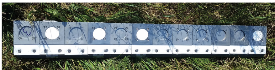
Figure 3. A row of passive samplers fixed on a holder bar, ready for installation in river water and hyporheic sediments.
