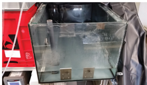
Figure 6. Stagnant water conditions were simulated using an aquarium.
