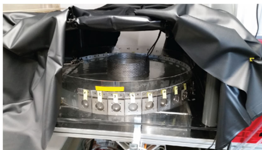
Figure 5. Circular flume used for method validation.
