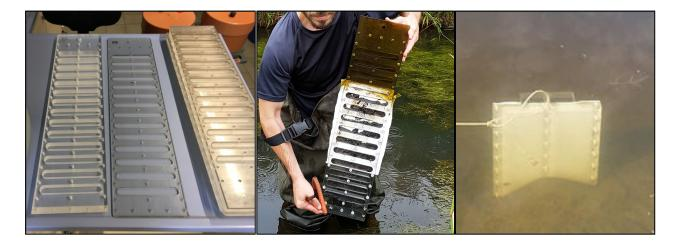
**Figure 1.** Left: Parts of the dialysis sampler (peeper). Middle: Image of the peeper after piercing the dialysis membrane. Right: Peeper installed in the riverbed.
